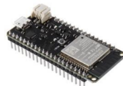
Gambar 2. lolin ESP 32 VROOM 32D
